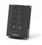
The *PowerPlex®* PM500 includes a physically isolated CAN bus interface and redundant protective functions for connected DC loads. One power module can control and monitor a total of twelve electrical loads. Each module has a manual override function for each 8 A and 25 A output via integral electro-mechanical mini circuit breakers. This allows manual and direct switch-over and ensures access to critical functions.
